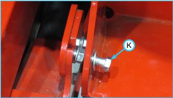
19. With the mounting bolts through the frame install the 3/8" flange nuts (L) to secure the seat in place, Torque the flange nuts to 31 ft-lbs (42 Nm).
