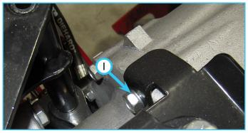
14. Remove the two 1/2" bolts (J) from the shifter mounting bracket.
