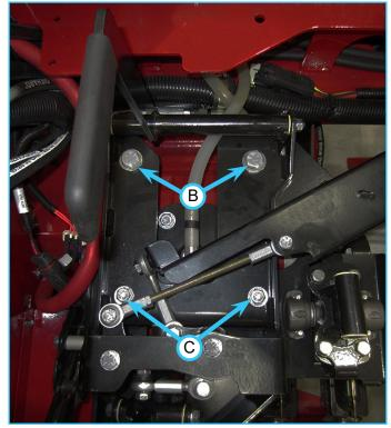
5. Install the two 3/8" mounting bolts (C) through the mounting bracket and into the two speed
